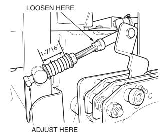
Figure 6-2. Brake Rod Adjustment
